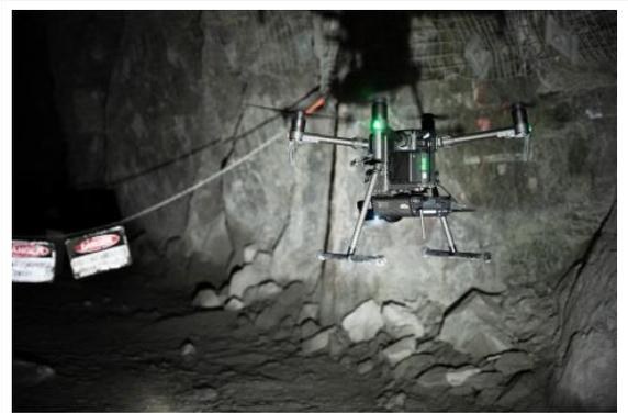
Emesent's Autonomy Level 2 (AL2) technology for Hovermap, using Velodyne's lidar sensors, enables companies to rapidly map, navigate and collect data in challenging inaccessible environments such as mines, civil construction works, telecommunications infrastructure and disaster response environments. (Photo: Emesent)
