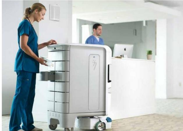
The robots come **equipped** with biometrically and PIN-locked drawers for secure equipment and sample transport, are self-charging (with up to 10 hours of activity between charges), and can carry up to 1,000 pounds.
